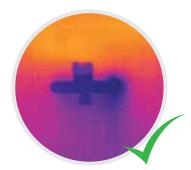
Mixing tap connected using a thermal separator. (Temperature < 25 °C in the PWC drop ear elbow)
