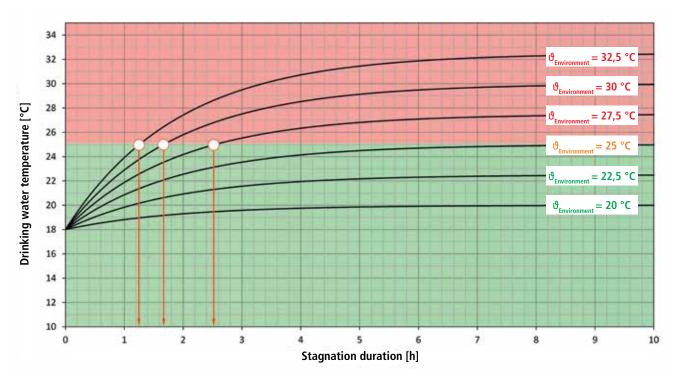
Temperature curve of a stagnant, 100 % insulated drinking water pipe made of copper (22 x 1.0) at different ambient air temperatures
