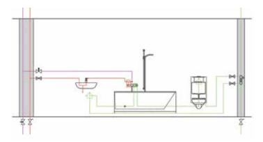
Heat transfer must be avoided at the design stage by laying hot pipes and cold-water pipes separately.
