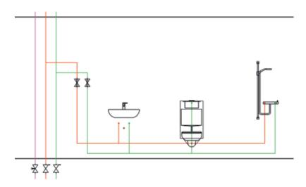
Standard T installation in the bathroom. Stagnation areas with a high risk of contamination arise when there are infrequently used tapping points.
