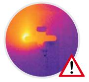
Mixing tap connected using double drop-ear elbows. (Temperature clearly > 25 °C in the PWC drop ear elbow)
