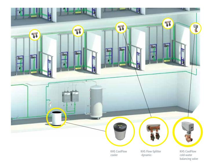
With the addition of KHS CoolFlow in the innovative KEMPER Hygiene System KHS, cold water temperatures of less than 20 °C can now be permanently achieved up to the tapping point. The drinking water is distributed to the tapping point via a KHS Flow-Splitter. The KHS CoolFlow cooler cools and circulates the drinking water. The KHS CoolFlow cold water balancing valve regulates, flushes and shuts off circulation circuits as required.
