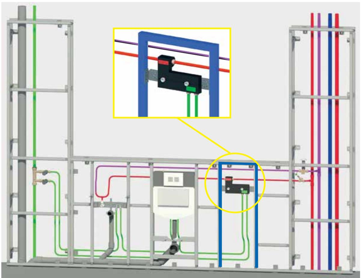
Example of a bathroom in a building with special hygiene requirements
