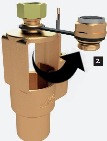
2. Remove the unscrewed gunmetal part from the KHS drain to the front and loosen it from the elastomer strap.
